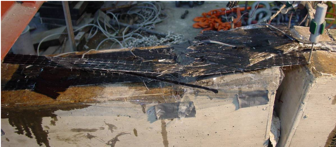
After Testing: Failure by FRP fracture
