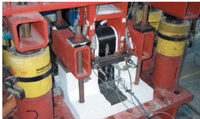
Figure 3-26 Shear test of carbon fiber anchor [Burr, 2004]
