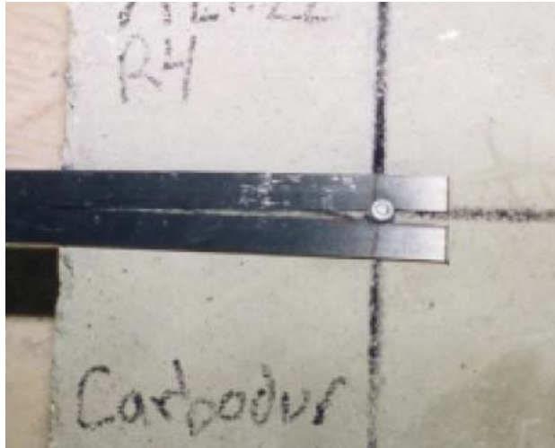
Figure 3-16 Splitting failure of prepeg plate with unidirectional fibers [Lamanna, 2002]
