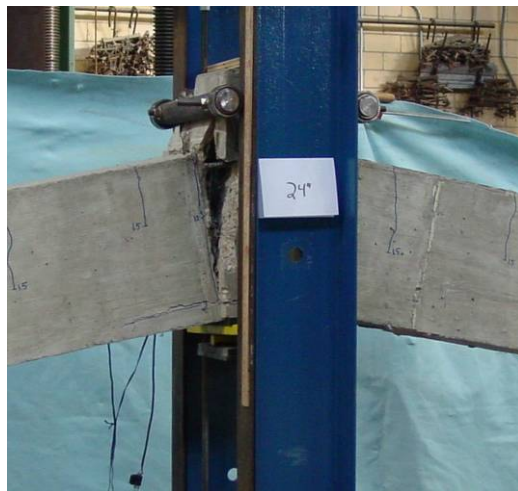
Figure 5-40 Wide crack and pulling out of #3 bars at column line
