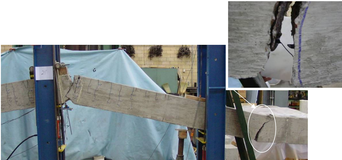
Figure 5-67 Fracture of negative moment rebar
