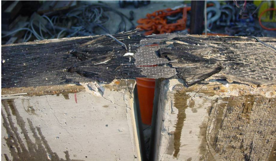
Figure 4-21 Failure by CFRP fracture for retrofit with two larger anchors per row (00-4s3)
