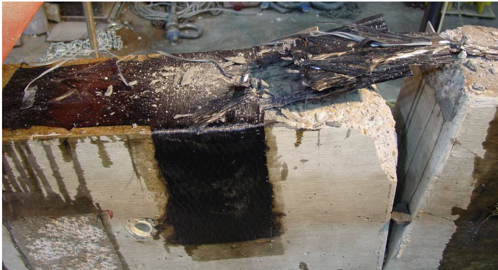
After Testing: Failure by FRP fracture
