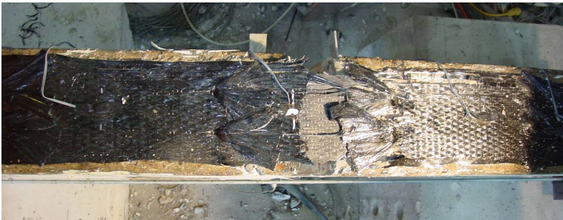
After Testing: Failure by FRP fracture
