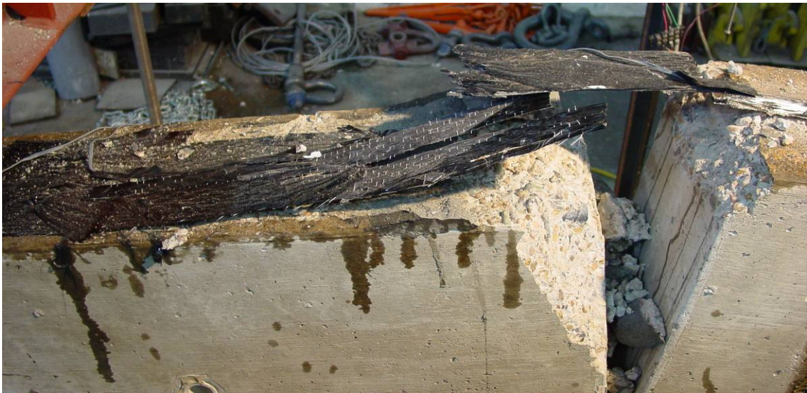
After Testing: Failure by FRP fracture
