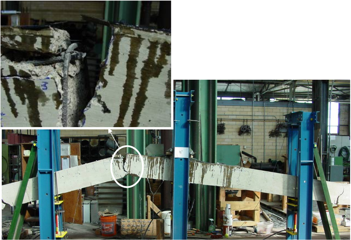
Figure 5-25 Failure of PM-1 by fracture of rebar
