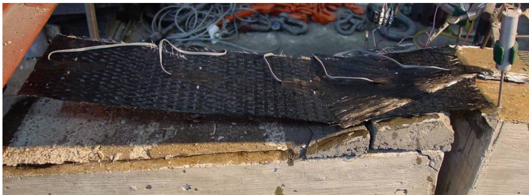
After Testing: Failure by debonding
