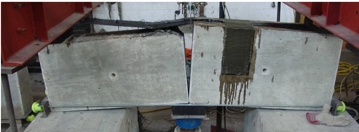
After Testing: Failure by debonding
