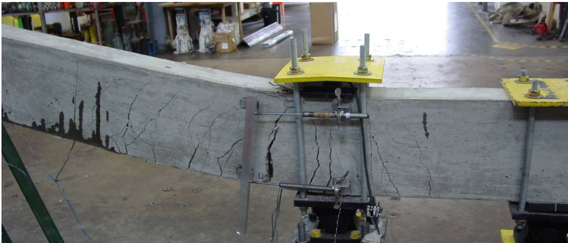
Figure 5-52 Distributed cracking in hinge region
