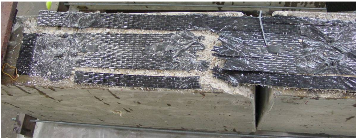
After Testing: Failure by partial debonding and fracture
