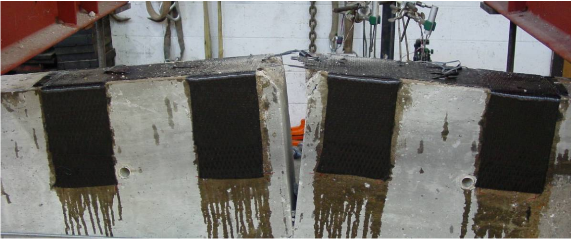
Figure 4-16 Failure by FRP fracture of retrofit with double layer U-wraps (00-us2)
