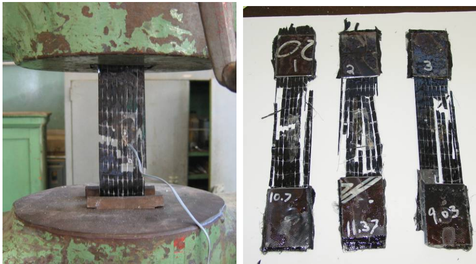
Figure 4-10 FRP coupons tested in accordance with ASTM D-3039
