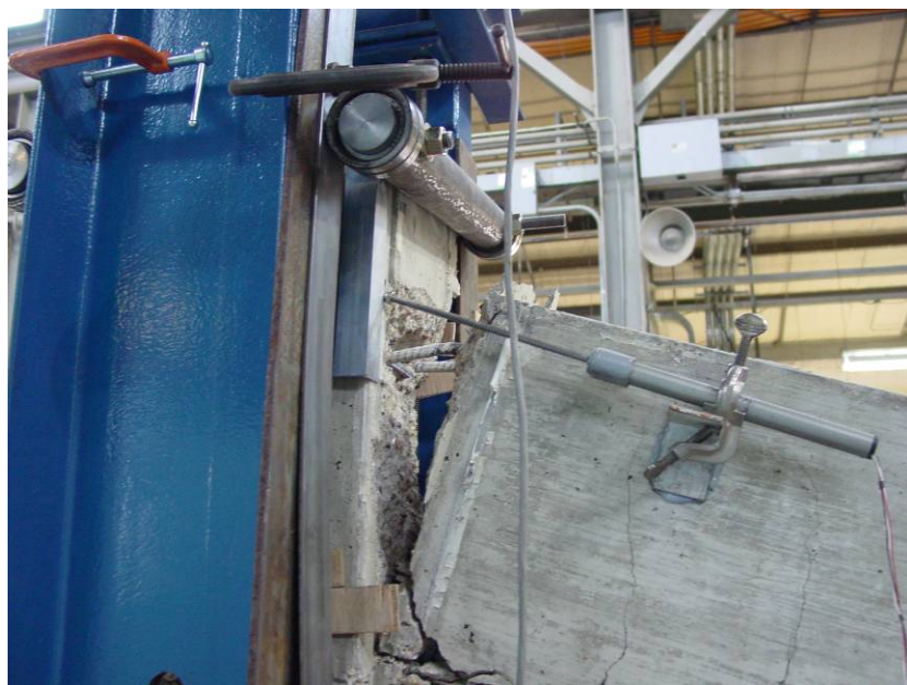
Figure 5-53 Linear pot to measure crack opening
