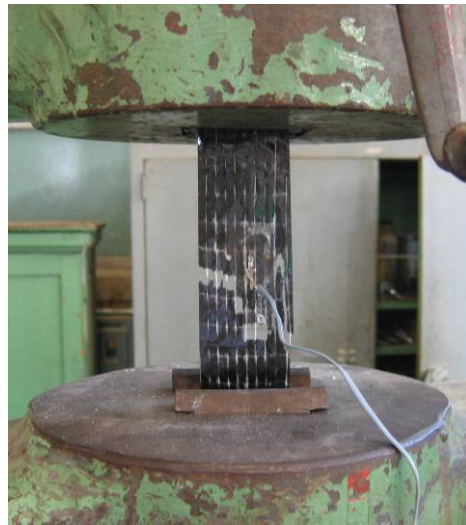
Figure 3-8 CFRP coupons in hydraulic testing machine
