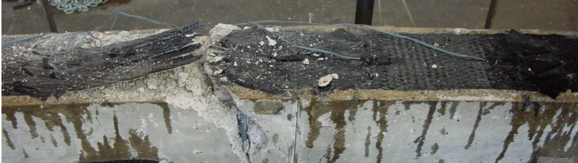
Figure 4-19 Failure by FRP fracture of retrofit with three anchors per row (00-6s1)
