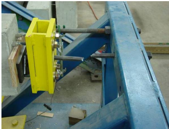
Fracture of threaded rod for axial restraint
