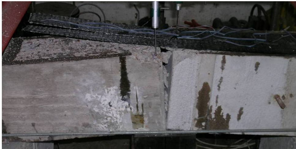
After Testing: Failure by Debonding
