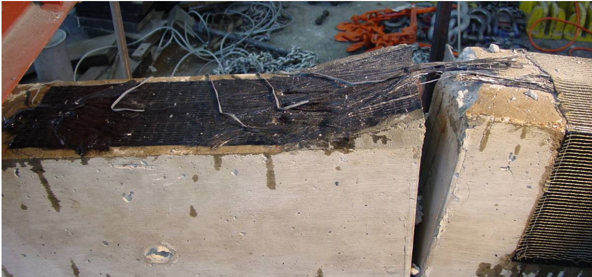
After Testing: Failure by FRP fracture
