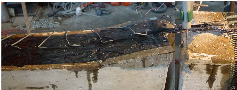
After Testing: Failure by FRP fracture of column bundle
