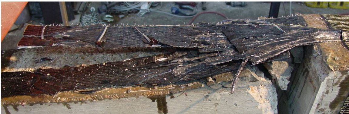
After Testing: Failure by anchor fracture
