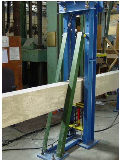
Figure 5-16 Braces (green) to provide lateral restraint and support North and South blue columns
