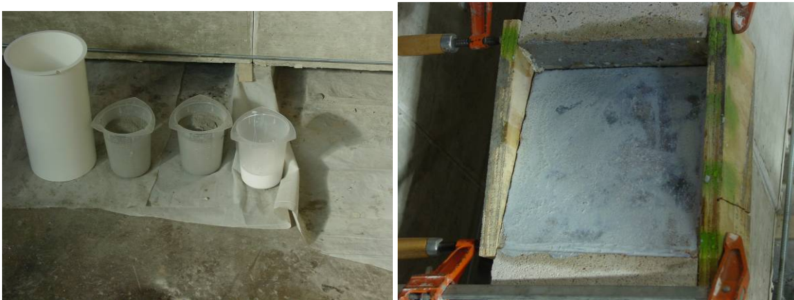
Figure 3-33 Repair material components and painting of concrete with latex solution
