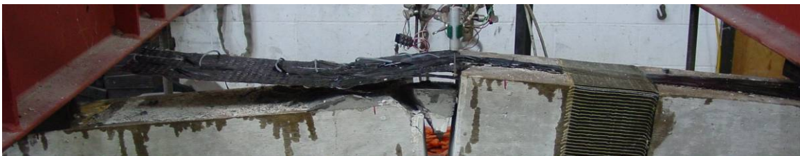
After Testing: Failure by anchor fracture
