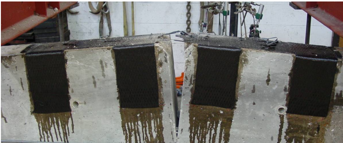
After Testing: Failure by FRP fracture
