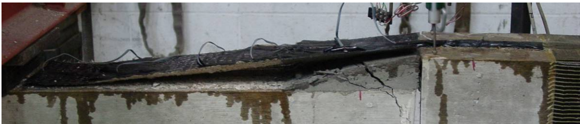
Fracture first row of anchors
