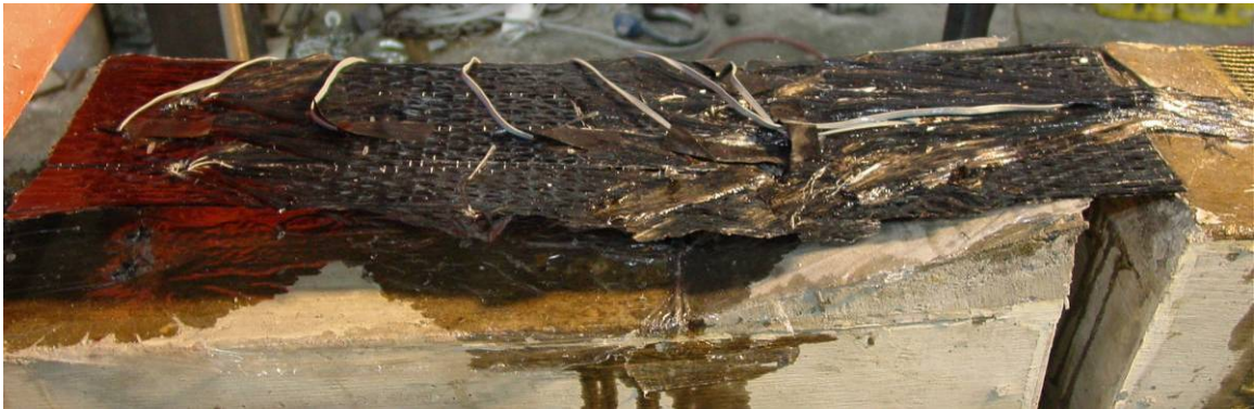
After Testing: Failure by anchor fracture
