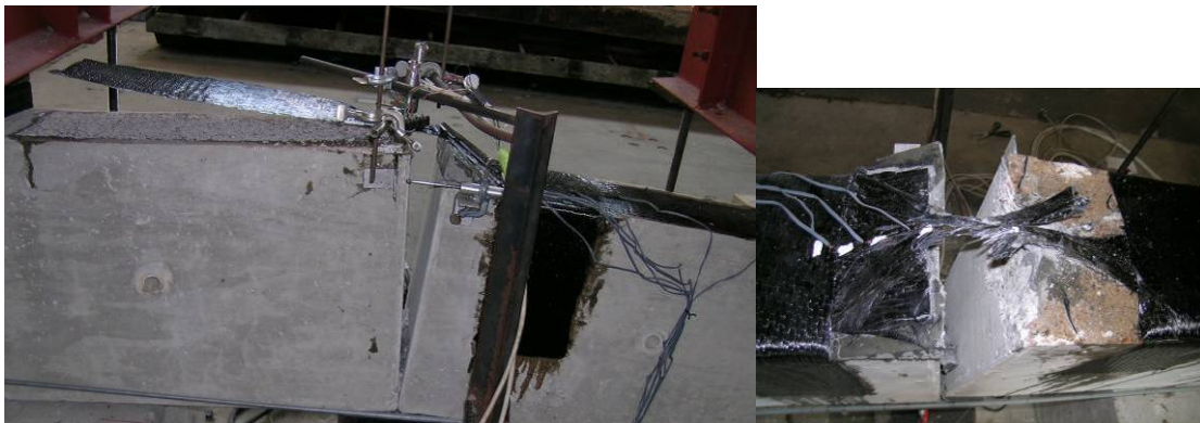
After Testing: Failure by Debonding, After Retest by FRP Fracture
