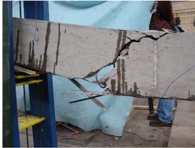
Figure 5-57 Fracture of negative moment CFRP
