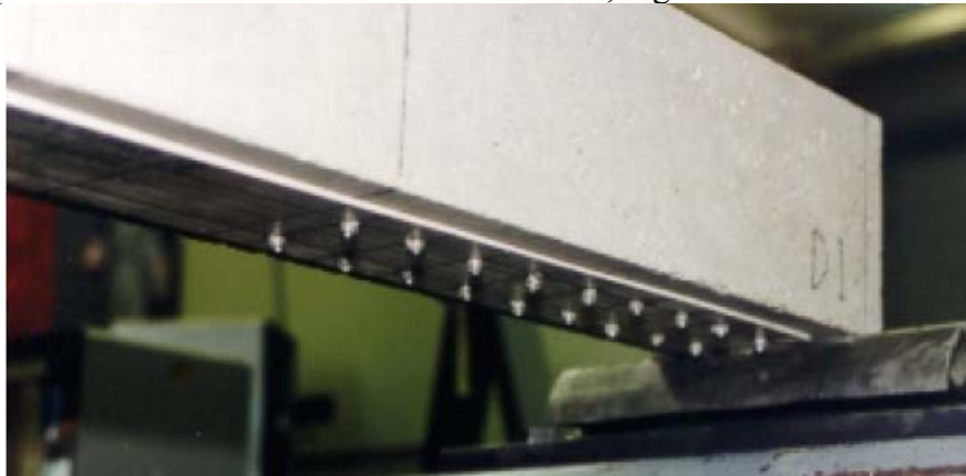
Figure 3-15 Mechanical fastening of prepeg CFRP plate [Lamanna, 2002]
