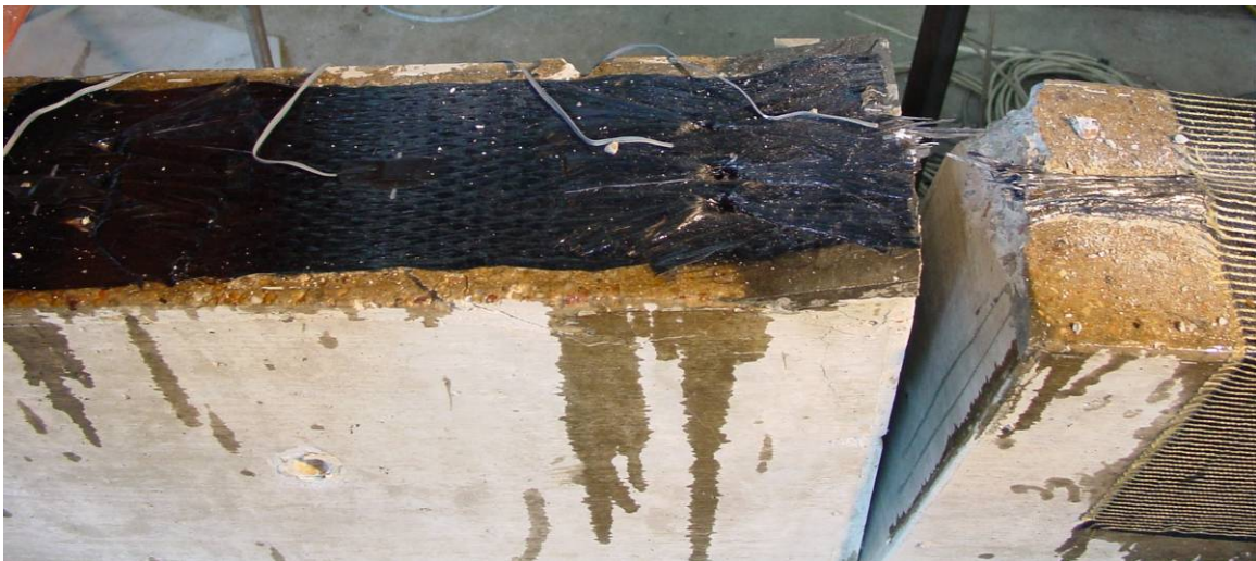
After Testing: Failure by FRP fracture
