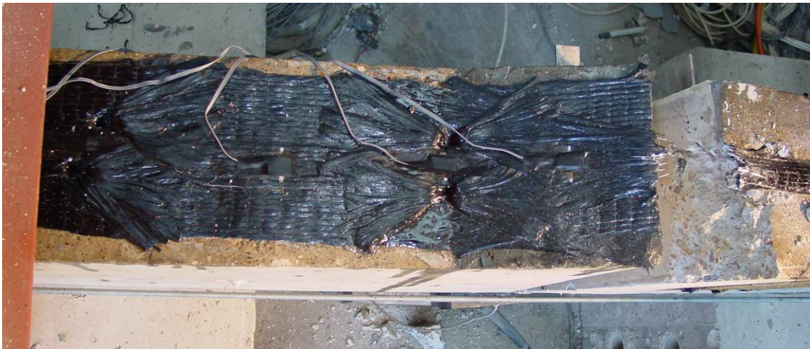
After Testing: Failure by FRP fracture
