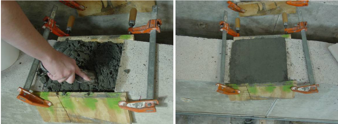
Figure 3-34 Placing and leveling of ramp material
